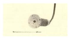
Model 410: LVDT coil is housed in a metallic cylindrical tube with collet type cable assembly at one end for drawing out the sensor cable and flange with three holes to facilitate fixing of transducers at other end. The core is held in a mandrel i.e., the core is fixed to the object whose movement is required.
